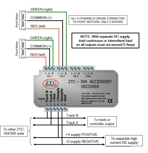
For solenoid point motors the ZTC 304 must be used. It is also recommended that, if a capacitor discharge unit is not available, an external regulated high current DC power supply must be connected to reduce the load on the track feed voltage. The external power must be regulated DC only.
