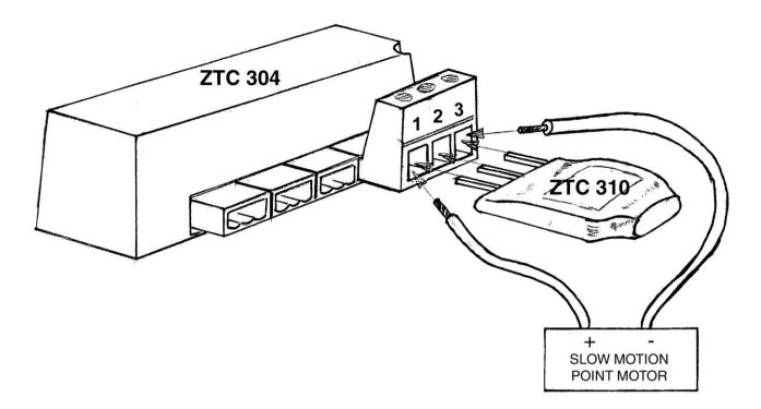
One end of the ZTC 310 has 3 pins for connecting to the accessory decoder. The pins are spaced to fit in the existing screw terminals on the accessory decoder plug. This makes installation extremely simple.
