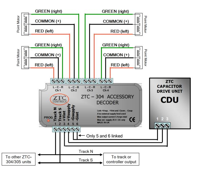
Using a capacitor discharge unit (CDU) allows solenoid point motors to be powered from
