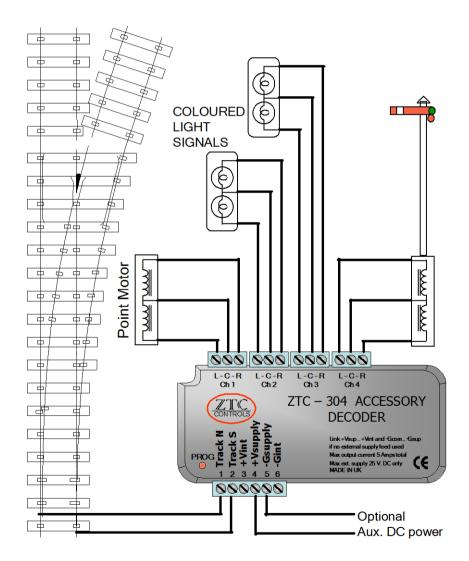
The ZTC 304 has power output drivers capable of direct operation of large solenoid point motors drawing up to 8 amps. The ZTC 305 will drive loads up to 0.5 amps and is more suitable for light signals and other low current applications.
