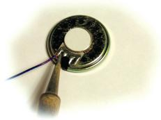
Figure 18 - Soldering to the Speaker Terminals
