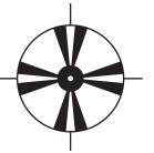
For simple articulated engines, a synchronizer disk is available that provides 8 chuffs per driver revolution.
